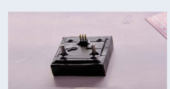
Figure 26: SiPM PCB and scintillator wrapped in electrical tape.
